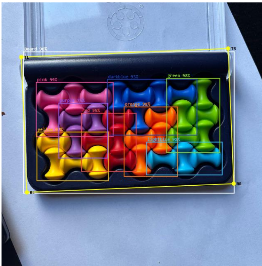
Figure 7: Board corner detection showing the four corners (TL, TR, BL, BR) identified from the board's segmentation mask.
