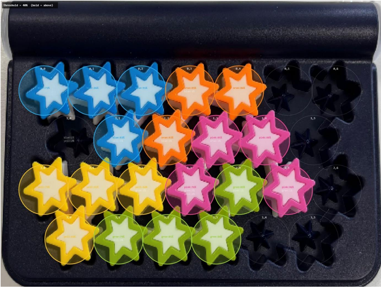
Figure 37: Grid mapping on IQ Stars, showing the circular cell regions and cell coordinates on a perspective-corrected board.
